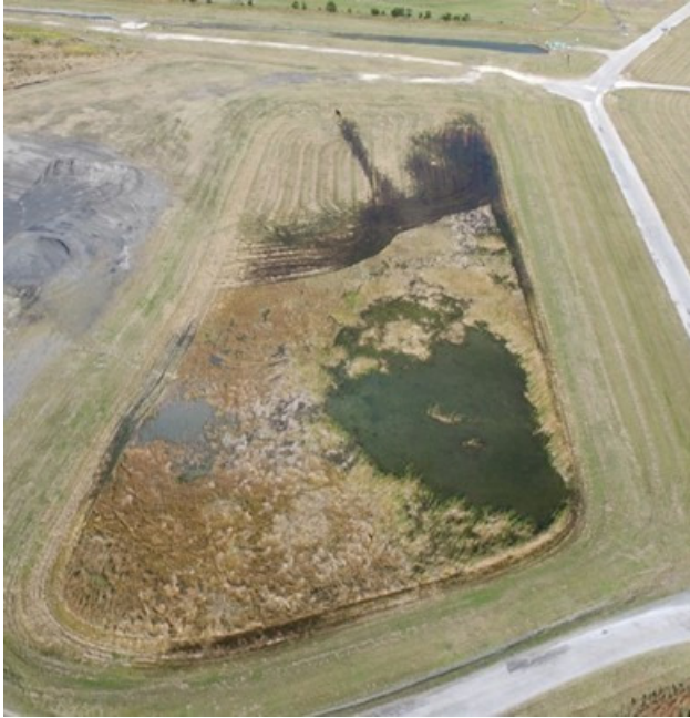
Figure 13. Aerial Image of Ponding in the Southern End of the Cell 4 Basin Area
