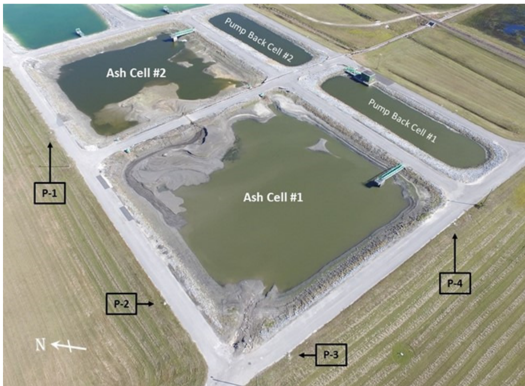
Figure 1. Layout of the CCR Surface Impoundment System and Adjacent Pump Back Ponds (IWCS 2017a)
